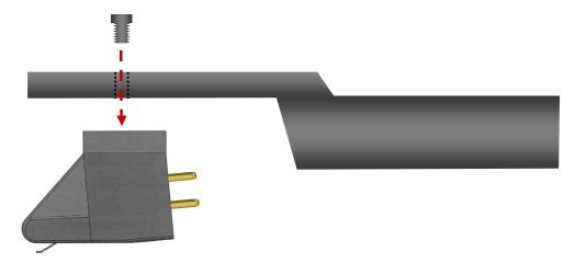
Once the cartridge is in place, set the correct tracking weight. Do this BEFORE the final adjustments are made for cartridge alignment, as this will help to ensure the cantilever is not damaged due to excessive tracking force. Once final alignment adjustments have been made, it will be necessary to check the tracking weight again, as any movement of the cartridge body will change the tracking weight.
