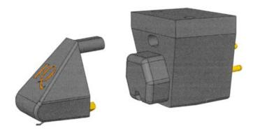
To protect the stylus from damage during installation, we recommend removing the stylus assembly from the cartridge body, as in the above illustration.
